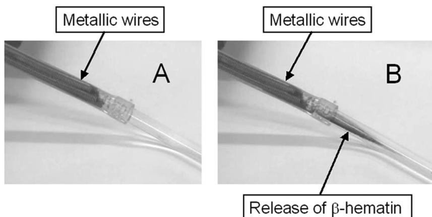
Fig. 2. Trapping and elution of  $\beta$ -hematin (A)  $\beta$ -hematin trapped on metallic wires (magnet removed; flow off) (B) Elution of  $\beta$ -hematin (magnet removed; flow on).
